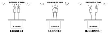
It is recommended that the IR sensors are mounted under your layout and pushed up between the sleepers in the centre of your track. Drill two 4.0mm (5/32 inch) holes with 5mm between their centres or make a 4.0mm x 9.0mm slot, being careful not to damage the track. Screw the IR sensor in place, adding a spacer if necessary so that the top of the IR sensor sits level with the top of your ballast or sleepers.
